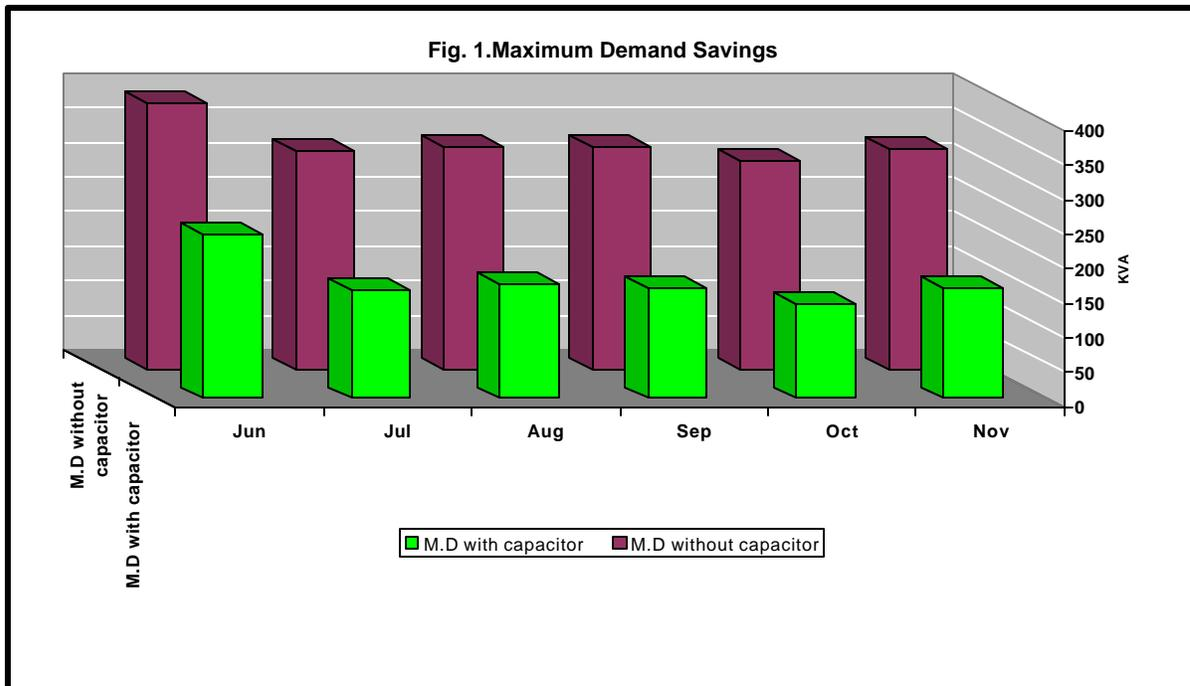
Fig.1 & 2 show that the factory's demand for electricity and cost is now much lower than it would have been without the capacitor bank. In spite of the additional
